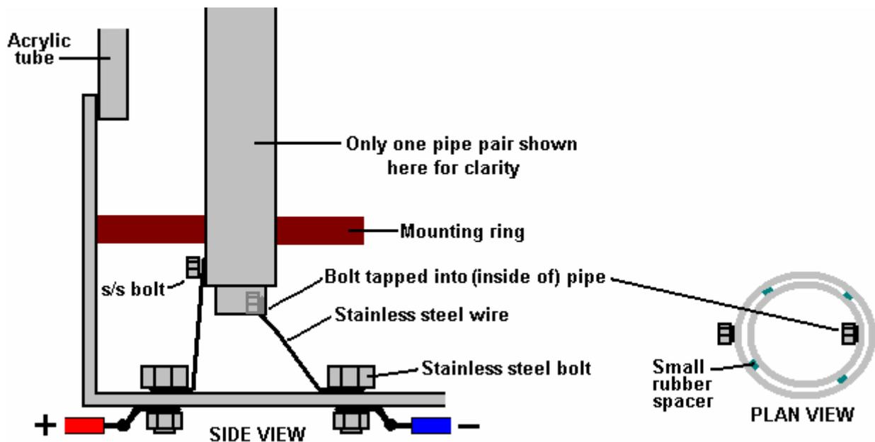
The bolts tapped into the inner tubes should be on the inside and the bottom of the two tubes aligned in spite of them being spread out as shown above. The diagram shows the inner connection on the outside, only for clarity. The bolts going through the base of the unit should be tapped in to give a tight fit and they should be sealed with Sikaflex bonding agent or some similar waterproofing material.
