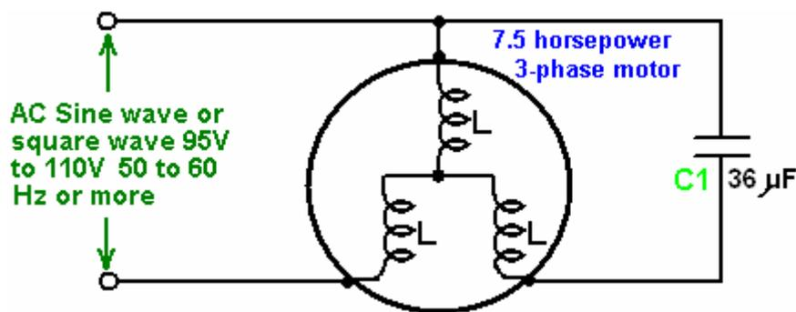
Because the running power draw is so low, it is possible to run this motor from a standard battery-powered inverter, but the current draw at start-up is some 17 amps, so the mains is used to get the motor started and then the motor is switched from the mains to the inverter. The inverter also allows easy measurement of the power input and so makes for easier calculation of the overall power efficiency of the system.
