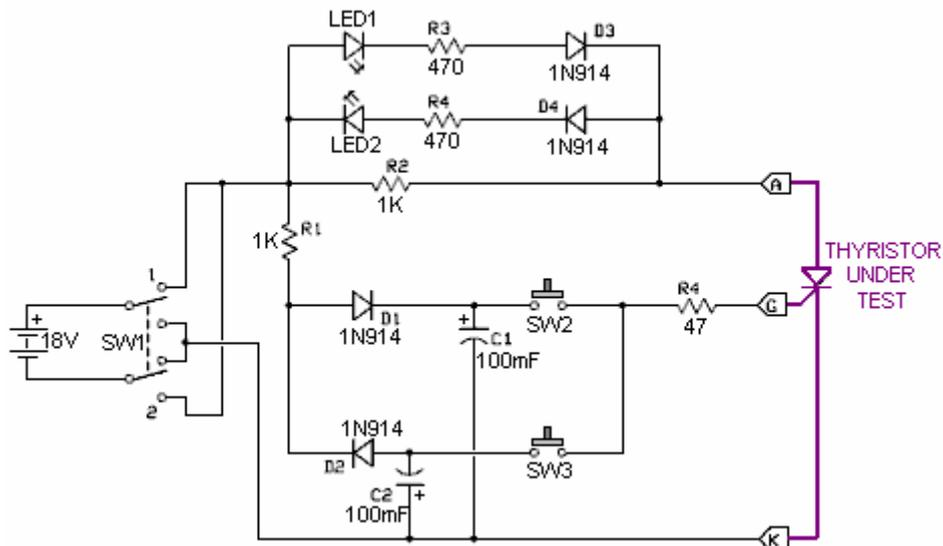
The circuit is operated by operating SW1 several times so as to get capacitors C1 and C2 fully charged. LED1 and LED2 should both be off. If either of them light, then the thyristor is faulty.
