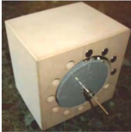
The housing has considerable clearance for the drum and magnets. The rear shaft bearing is just set into the back of the housing:
