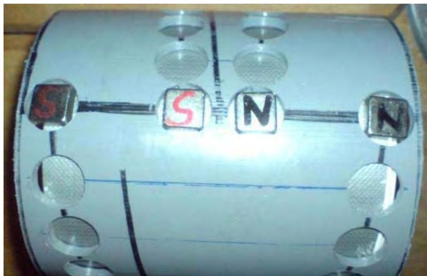
With Dietmar's design using angles magnet pairs, the number of magnets needed is quite high. For a single V, there are 58 magnets. For a 2-V version, 106 magnets. For a 3-V version, 154 magnets and for a 4-V version, 202 magnets if there is only one stack of stator magnets, so ten extra magnets need to be added to the count for
