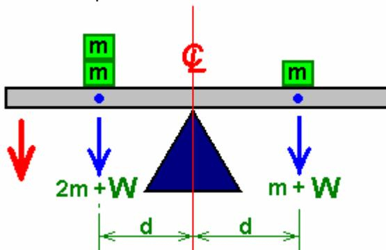
With this unequal loading, the beam will tip down on the left hand side, as indicated by the red arrow. This seems like a very simple thing, but it is a very important fact. Let me point out what happens here. As soon as the weight on one side of the pivot is bigger than the weight on the other side (both weights being an equal distance from the pivot point), then the heavy plank starts to move. Why does it move? Because gravity is pushing the weights downwards.
