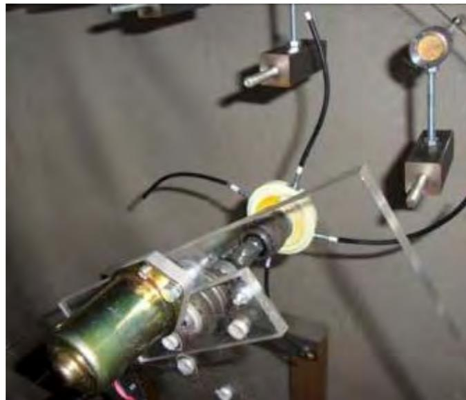
Each weight is held rigidly and so when the motor arm presses against it, the lever arm is pushed out sideways without the weight twisting away from the motor arm. These prototype weights are not heavy, but when a working unit is being built they will have considerable weight, so to get a well balanced arrangement, it might be advisable to have weights on both sides of the wheel so that there is no offset axial load placed on the shaft which supports the wheel:
