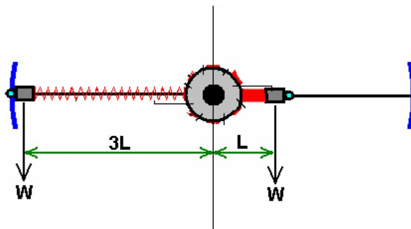
Take any one weight for this calculation. Any excess rotational energy will be created by the difference between the forces attempting to turn the wheel in a clockwise direction and those forces trying to turn the wheel in a counter-clockwise direction. For the purpose of this discussion, let us assume that we have built the wheel so that the compressed-spring position is one third of the spring-uncompressed position.
