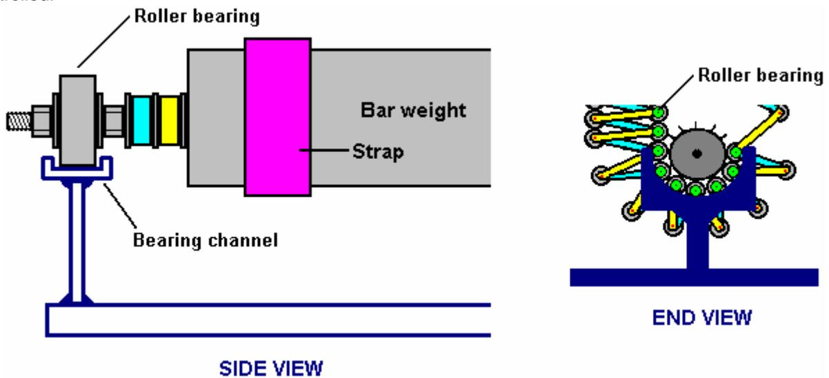
A guiding channel can be used, as shown here, and standard ball-bearings or roller-bearings can be attached to the ends of the weights by using threaded rod (or a bolt with the head inside the weight) and locking nuts.
