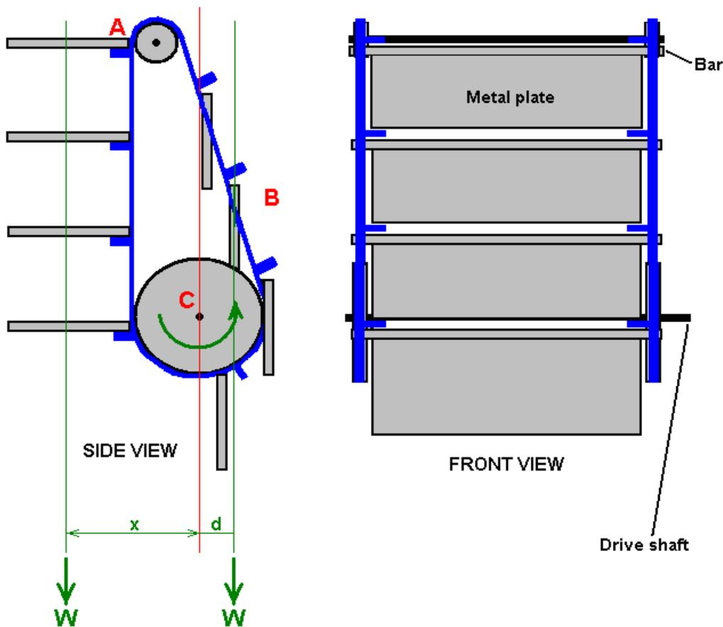
This design uses heavy metal plates which are carried on two drive belts shown in blue in the diagram above. These plates are hinged so that they stand out horizontally on the falling side, resting on a pair of lugs welded to the chain link and hang down vertically on the rising side as they are narrower than the gap between the belts.
