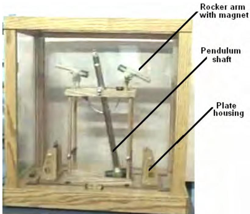
The device operates like this: The pendulum swings to the right and as it does so, it raises a magnet attached to the pendulum shaft by a curved silver arm:
