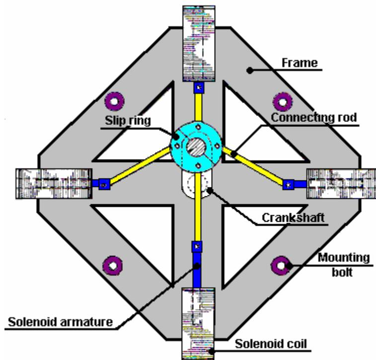
This style of motor is simple to construct and yet very powerful. The switch for each solenoid can be a very simple mechanical switch which is pushed closed by a cam when the crankshaft is in the position where the solenoid should pull, and opens again when the crankshaft reaches the position where the solenoid should stop pulling. This motor also meets the requirement for rapidly repeated impulses to the axle of the flywheel.
