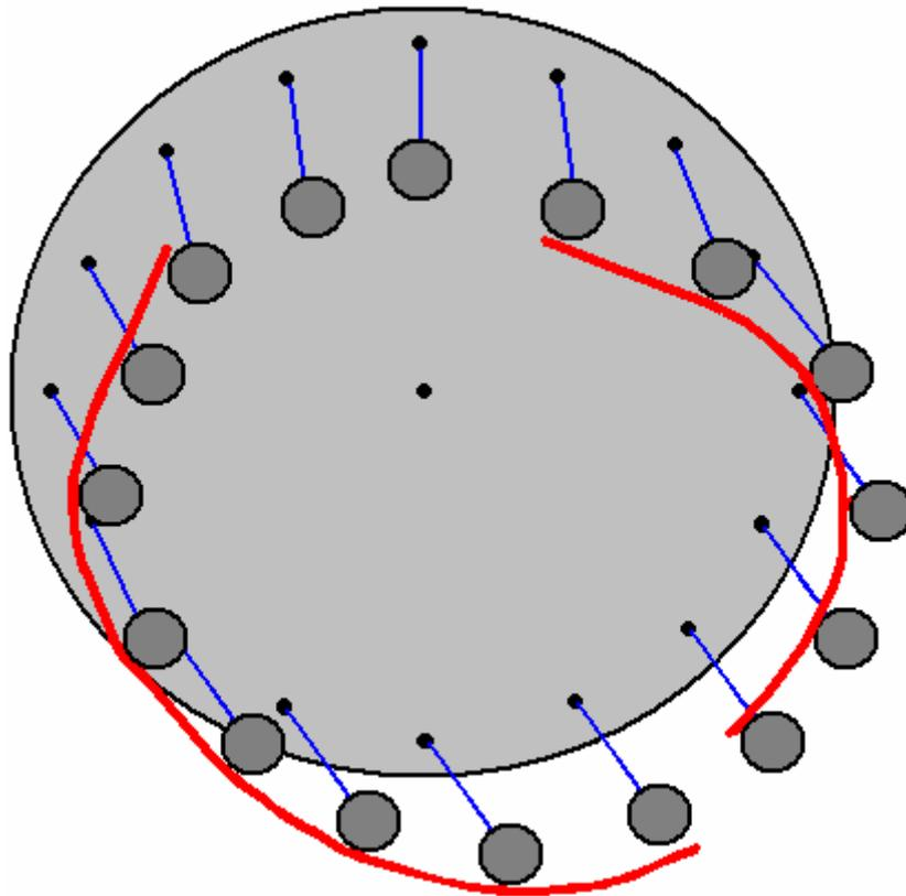
Admittedly, the deflector pieces would have a smoother shape than drawn here, but the principle is shown in spite of the poor quality of the diagram. Where heavy weights are involved, each would need to have a roller bearing pressing between the weight and the deflector shield in order to minimise friction as the weight slides past. A fairly similar idea is part of the next entry from Dale Simpson.
