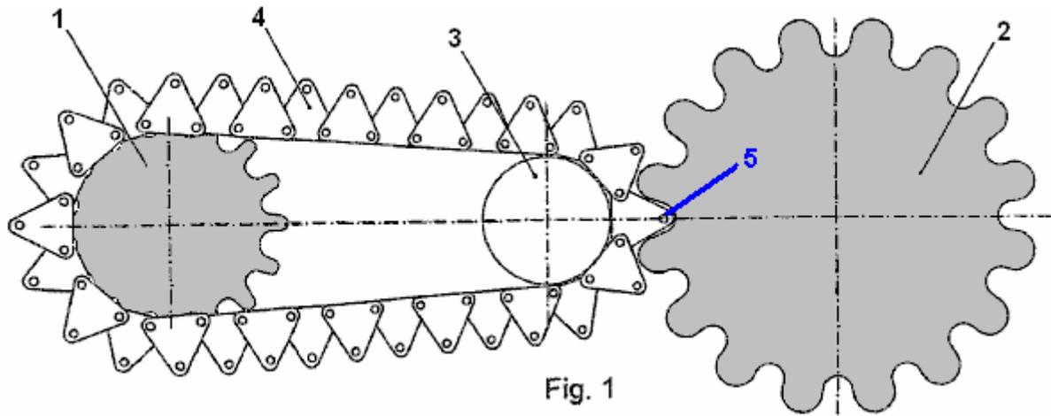
The way that the chain manages to push the larger teeth of the large wheel is by having the driving roller “5” raised by a triangular link “4” so that it has the same rotational pitch as the teeth on the larger wheel.
