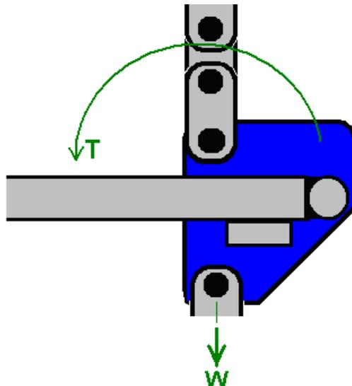
Where the weight of the plate acts directly downwards on the chain and there is a turning force “T” which does not contribute in any way to the driving force of the chain.
