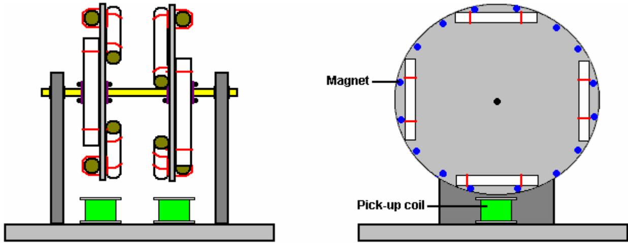
If the rotor spins well, then it would be worth while attaching a series of magnets to the discs, being careful to keep each disc perfectly balanced. One or more air-core coils can then be used to determine if current can be drawn from the device without stopping the rotation. The coils should not have a magnetic core as that would cause a major drag on the rotation whether current was being drawn or not.
