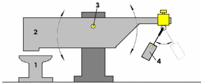
Here, the beam 2 is very much heavier than the pendulum weight 4. But, when the pendulum is set swinging by a slight push, the beam 2 pounds down on anvil 1 with considerable force, certainly much greater force than was needed to make the pendulum swing.
