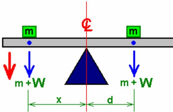
This is because the larger lever arm “x” makes the left hand weight “m” have more influence than the identical weight “m” on the right hand side.
