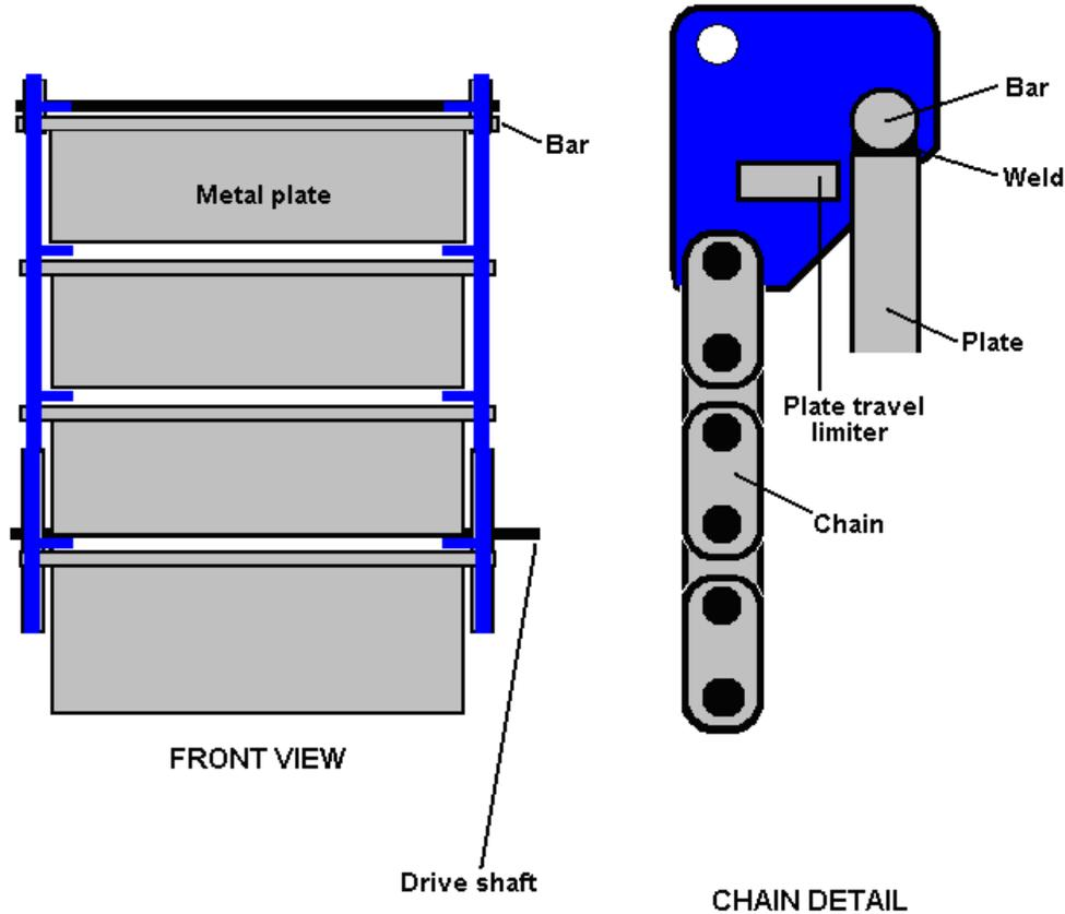
It should be noted that the movement of the lowest edge of the plates as they turn over when moving past the upper wheel at point “A”, is much faster than anywhere else, and so putting a protective housing around it would definitely be advisable as you don’t want anybody getting hit by one of these heavy plates.
