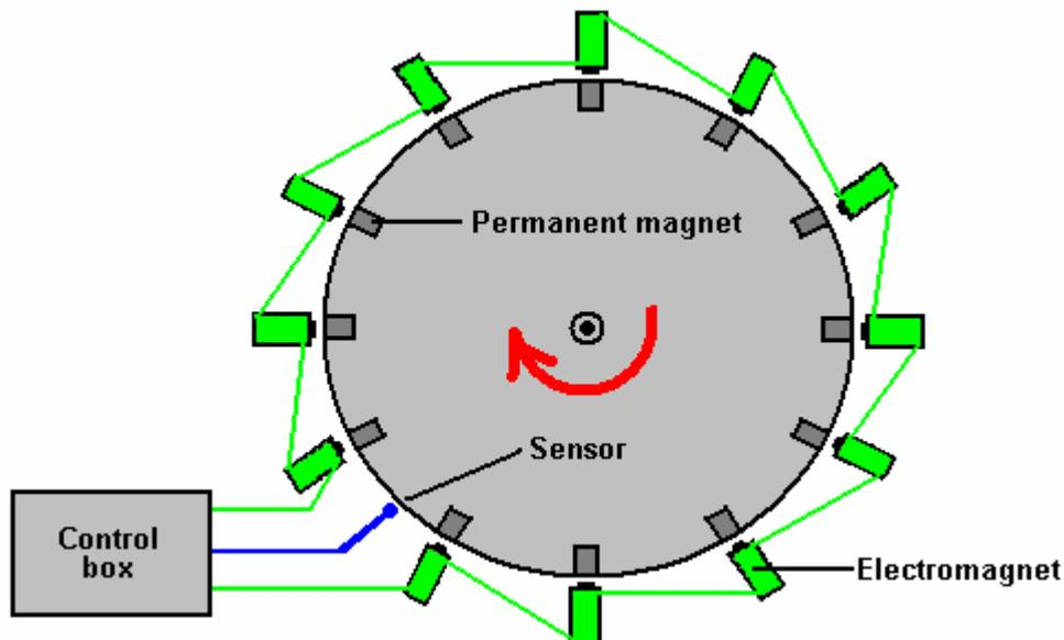
Here, the sensor generates a signal every time that one of the permanent magnets embedded in the rotor passes it. The control box circuitry allows adjustment of the time between the arrival of the sensor signal and the generation of a powerful drive pulse to the electromagnets, pushing the rotor onwards in its rotation. The control box can also provide control over the duration of the pulse as well, so that the operation can be fully controlled and tuned for optimum operation.
