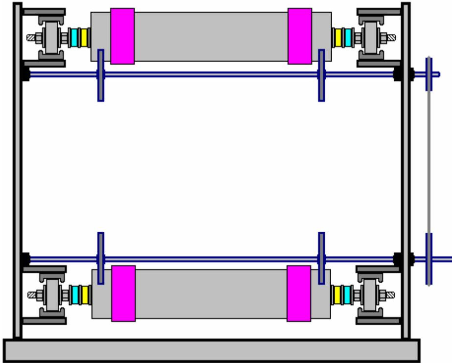
Here, the axel shafts are geared together outside the end wall and either a chain or a belt drive used. The lower shaft allows a power take-off. The ratio of the diameters of the pulley wheels or sprocket wheels dictates the relative rates of rotation of the two shafts.
