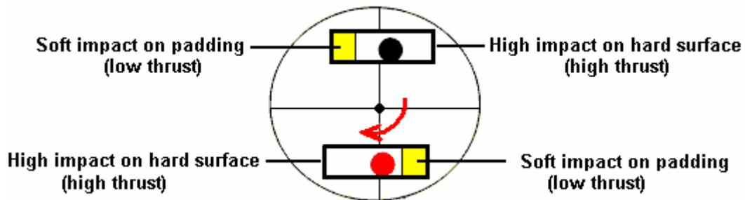
As the disc rotates, the ball falls down the length of the tube. At one end, the tube has a rigid cap which causes a significant impact when the ball hits it. The other end of the tube is padded and that cushions the impact which causes a net imbalance in the impacts and that maintains the rotation.
