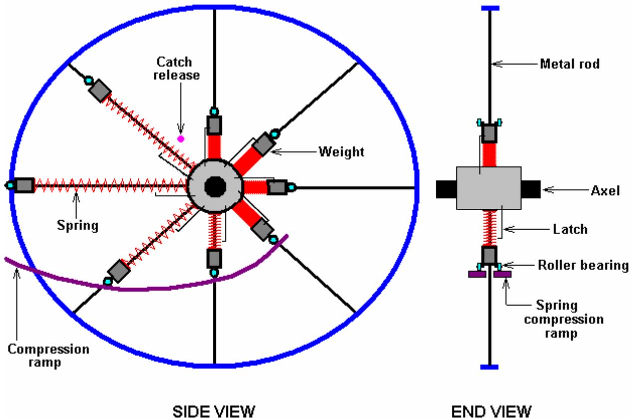
The wheel has an outer rim shown in blue and a central hub shown in grey. Metal spokes shown in black run out radially from the hub to the rim. Eight spokes are shown in this diagram as that number allows greater clarity, but a larger number would probably be beneficial when constructing a wheel of this type.
