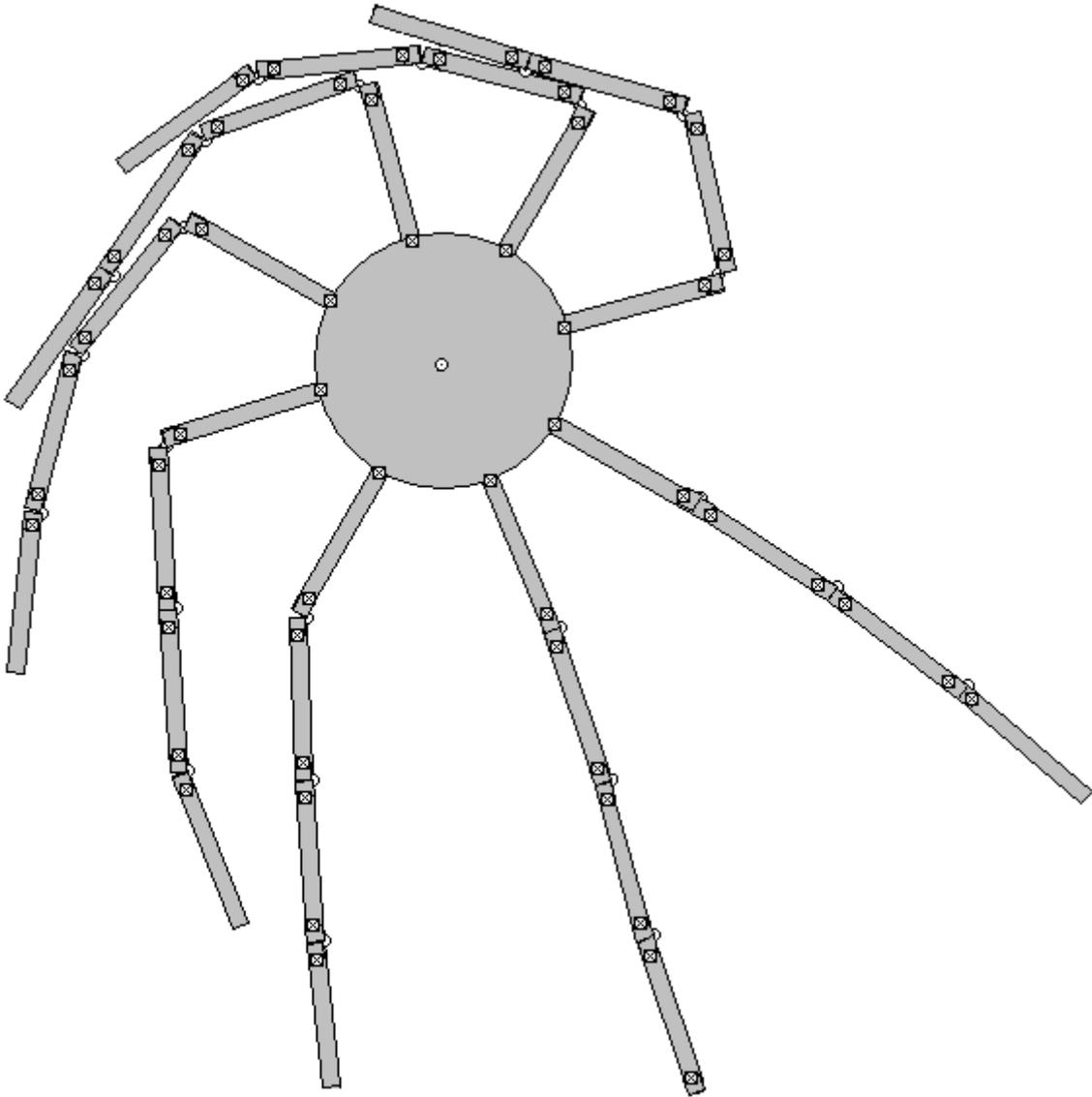
Here, the hinged arms or plates will also give an impact impulse when they open out to their full extent and that provides additional turning power. However, the imbalance between the two side is not a major amount and so this design is not likely to provide a large amount of torque for driving external loads.
