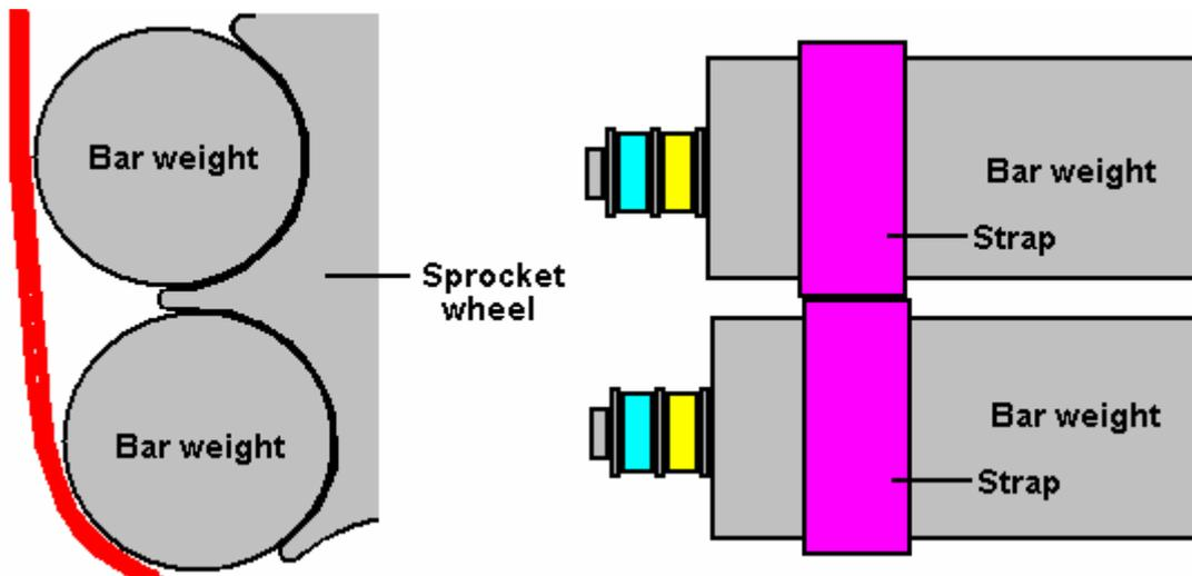
The description up to here has not mentioned the most important practical aspects of the design. It is now time to consider the rising side of the device. To control the expanded section of the chain, and to ensure that it feeds correctly on to the upper sprocket wheels, the gap between successive bar weights must be controlled.
