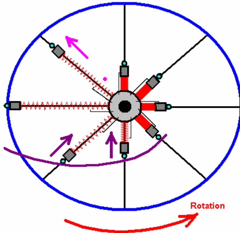
The question, of course is, will there be enough excess power to make the wheel rotate properly? The quality of construction is definitely a factor as things like the friction between the weights and their spokes needs to be very low. Let us consider the forces involved here:
