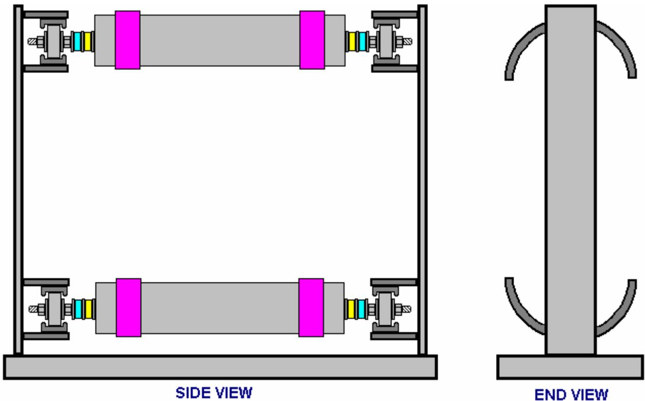
This method provides a low-friction channel for the roller-bearings to move along. This controls the position of the weights very accurately and the end walls also provide the supports for the axels which synchronise the positions of the weights and provide gearing between the axels if that is required. For clarity, just two of the many weights are shown and the overall proportions distorted so that the diagram will fit on the page.
