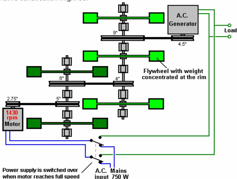
Here, there are five heavy flywheels mounted on two heavily supported strong axes, and while the two shown in dark green are only rotating at half the speed of the other three, the energy gain will be equal for each flywheel as each receives the same train of drive pulses. However, the pulley sizes might be better chosen in accordance with Jacob’s observations mentioned below.
