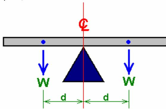
It balances because the weight of the plank ("W") to the left of the support point tries to make the plank tip over in a counter-clockwise direction, while exactly the same weight ("W") tries to tip it over in a clockwise direction. Both turning forces are  $d$  times  $W$  and as they match exactly, the plank does not move.
