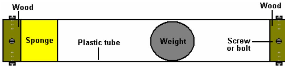
Here, a wood disc is fitted to each end of a piece of plastic tube and held securely in place with screws or bolts which pass through small holes drilled in the plastic pipe and screw into the wooden disc. A piece of thick sponge is glued to the disc at one end and the heavy weight inside the tube is not a tight fit so that it can move very freely inside the tube. Four of these tubes are fitted to each side of each disc used in the device as shown here:
