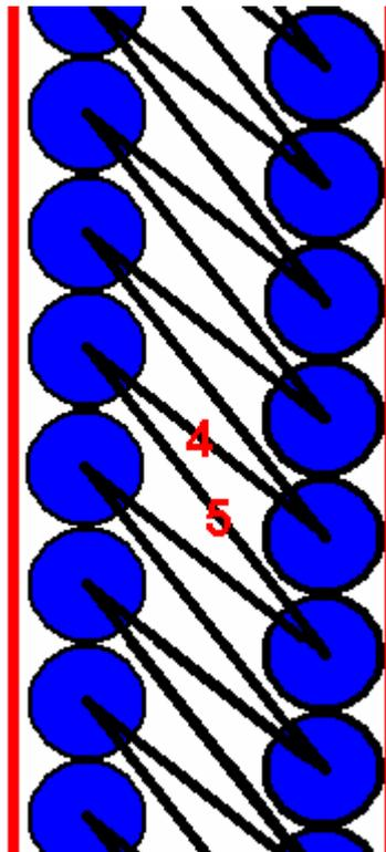
With this arrangement, the outer weights, shown here on the left, press down very firmly on the inside column of weights, making a compact group. If using plastic pipes with concrete then the hinge arrangement for the rods can be very simple, with a bolt set in the concrete as shown below.
