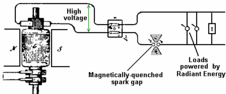
This was disclosed by Tesla in his 'Philadelphia and St Louis' lecture in 1893 and shows how loads can be powered when a high voltage source is pulsed by a magnetically-quenched sparks - this creates DC pulses of very short duration. More details about this are given in the accompanying document in this set entitled "D8.pdf" ('Devices' Part 8).
