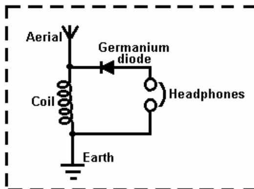
Looking at this in isolation, we appear to have a free-energy system which contradicts the Law of Conservation of Energy. It doesn't, of course but if you do not view the whole picture, you see a device which has only passive components and yet which (when the coil is of the correct size) causes the headphones to generate vibrations which reproduce recognisable speech and music. This looks like Energy Out with no Energy In.
