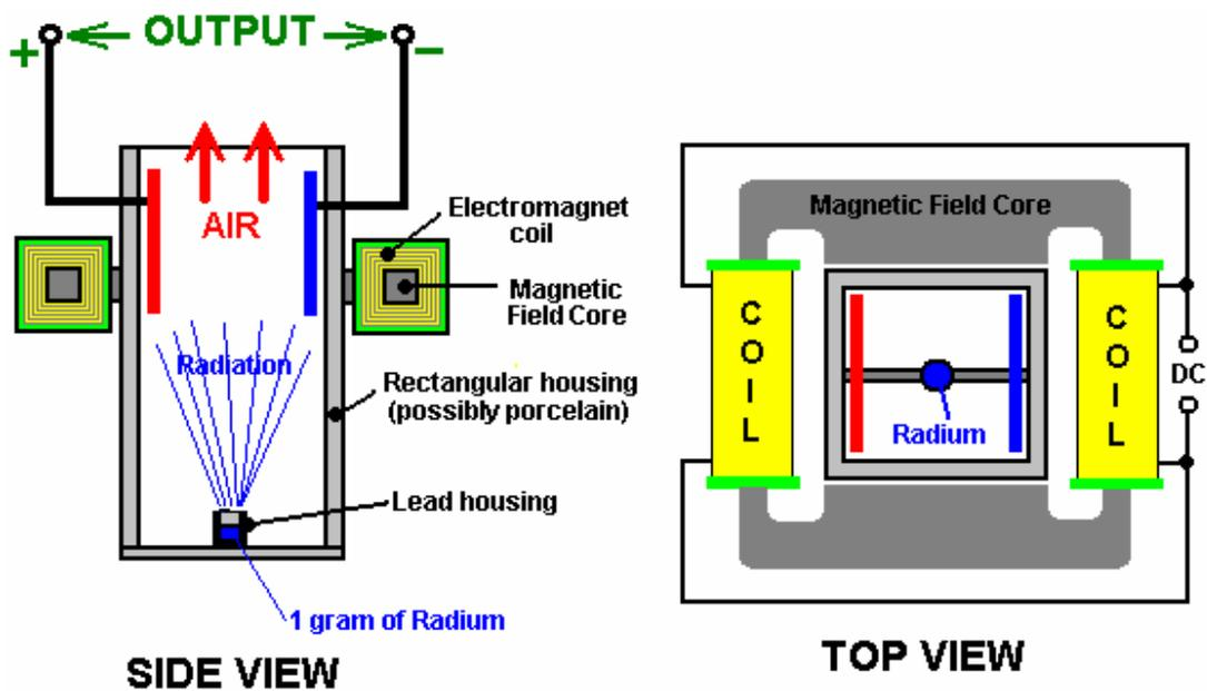
The variation of Tesla's device shown above, supports the lead container with its gram of radium on a strap across the bottom of the housing. The radiation ionises the air and the magnetic field separates the charges and directs them to opposite sides of the housing, to be collected and used via the electrode plates. There does not appear to be any reason why strong permanent magnets should not be used instead of the DC electromagnet shown.
