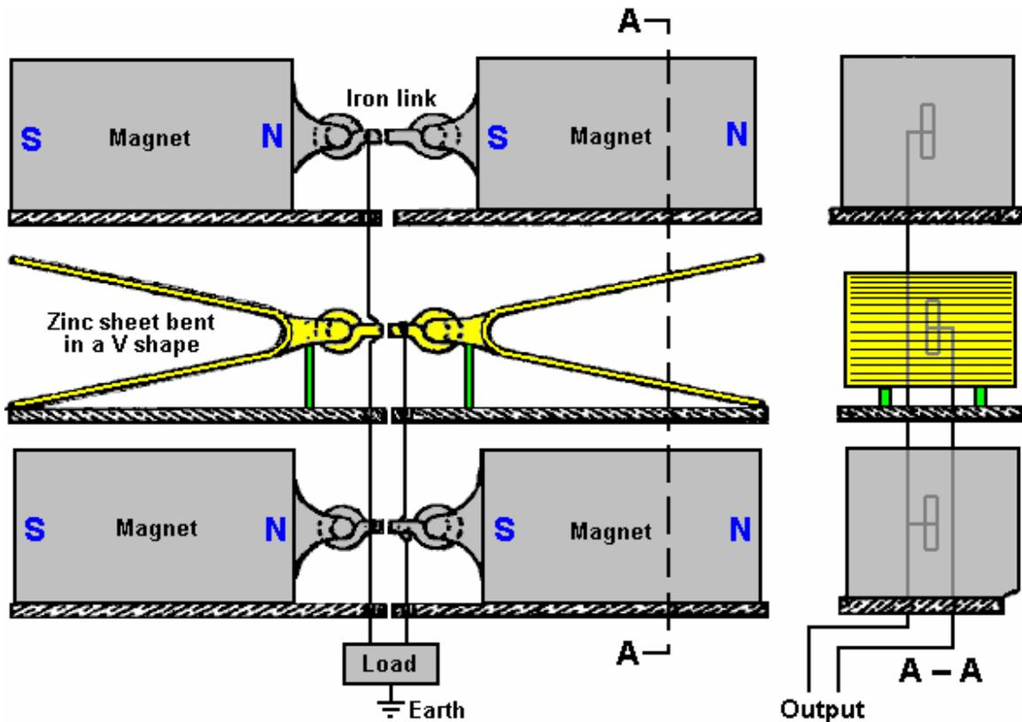
The zinc acts more effectively if installed as sheets bent into a V shape. The magnets and zinc sheets can be stacked vertically and/or horizontally and the greater the number used, the greater the electrical output. A good earth connection is recommended and presumably, the average cold water pipe of any house provides a more than adequate earth connection which is convenient to use.
