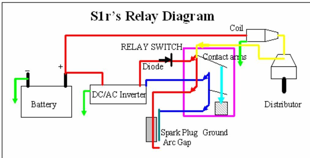
This is not an accurate depiction of S1r's relay as the wiring inside contained 4 diodes in an unusual configuration with dual solenoids, but it is indicative of the actual flow within the relay to the plugs.
