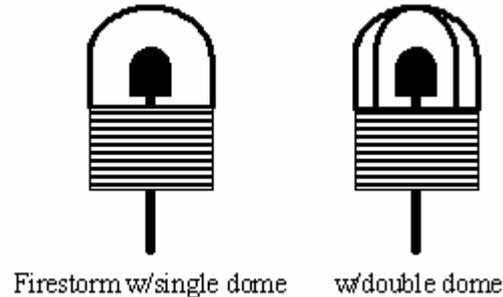
If these plugs ever come onto the market, they have very good potential for plasma fog jet engines as they create a plasma ball type explosion around the electrode. Till then you will have to make your own which could be done by welding a small dome onto the central electrode and then a wire dome over the top. Prototypes may not look that pretty, but they should work.
