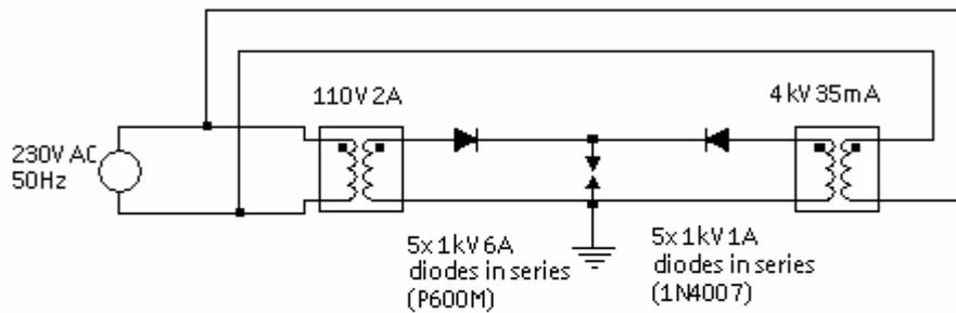
Diodes are used to isolate the sources. Note: both diodes need to withstand the HV if the HV source goes below 0V (AC source).
