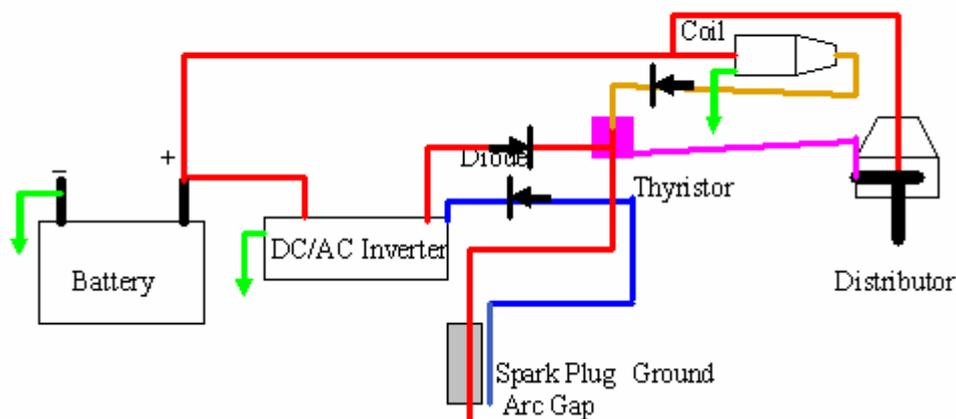
This same rotor-cap-thyristor approach can also be used in the inverter-diode-induction coil approach noted above as the triggering mechanism instead of using the traditional points. This approach would allow for the switching 'on' and 'off' of the inverter and coil circuits together and for a determined firing period or multiple periods.
