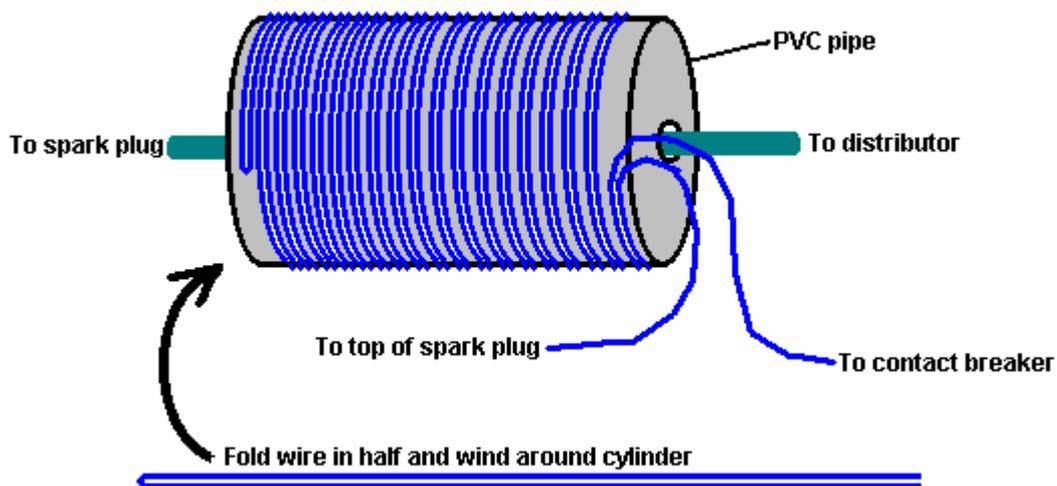
You can tape the wire in place on the cylinder. Now, run the spark plug wire through the cylinder to produce this arrangement:
