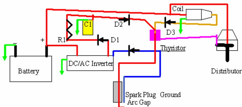
The above diagram is a modified CDI approach that uses the pulsed DC from the inverter to charge an electrolyte capacitor (C1) which is discharged through the thyristor when the circuit is opened by the distributor cap/rotor timing.
