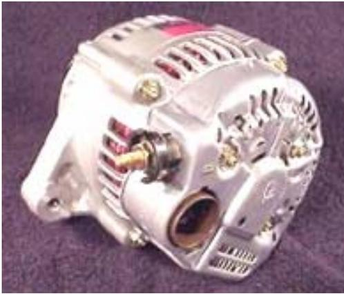
Most regulators are on the inside the alternator. Older models have externally mounted regulators.
