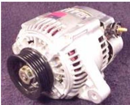
A vehicle charging system has three major components: the **Battery**, the **Alternator**, and the **Regulator**. The alternator works together with the battery to supply power when the vehicle is running. The output of an alternator is direct current (DC), however the alternator actually creates AC voltage which is then converted to DC as it leaves the alternator on its way to charge the battery and power the other electrical loads.
