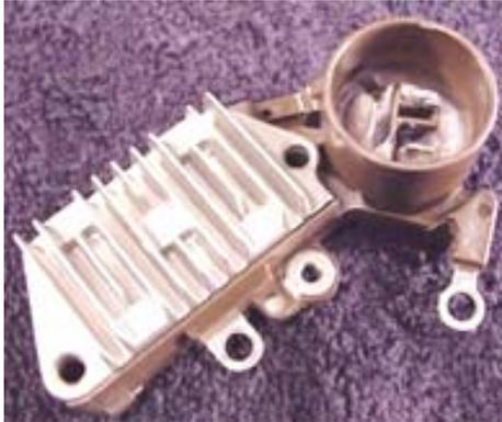
The regulator is the brain of the charging system. It monitors both the battery voltage and the stator voltage and, depending on the measured voltages, it adjusts the amount of rotor field current so as to control the output of the alternator.
