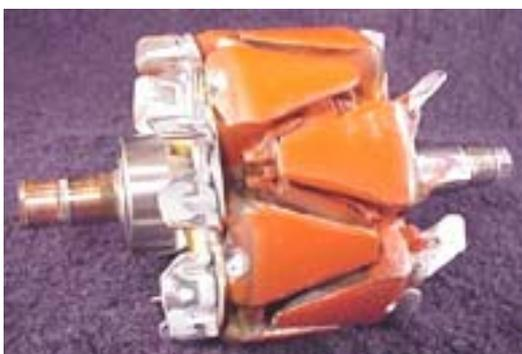
The rotor contains the field winding wound over an iron core which is part of the shaft. Surrounding the field coil are two claw-type finger poles. Each end of the rotor field winding is attached to a slip ring. Stationary brushes connect the alternator to the rotor. The rotor assembly is supported by bearings. One on the shaft and the other in the drive frame.
