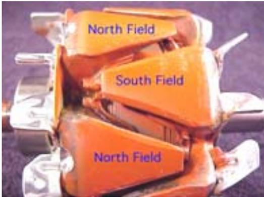
The rotor field winding creates the magnetic field that induces voltage in the stator. The magnetic field saturates the iron finger poles. One finger pole becomes a North pole and the other a South pole.
