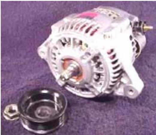
Alternator drive pulleys either bolt on or are pressed on the rotor shaft. Both 'V' and Multi-groove types are used. Please note this alternator does not have an external fan as part of the pulley assembly.
