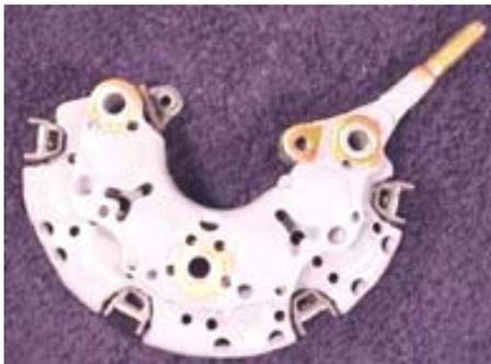
The **Diode Rectifier Bridge** is responsible for the conversion or rectification of AC voltage to DC voltage.
