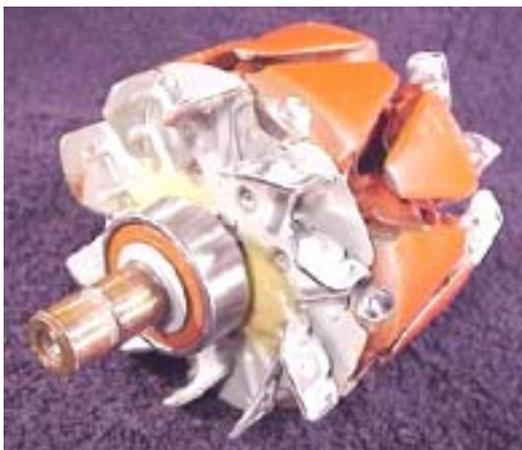
A basic rotor consists of an **iron core**, a **coil winding**, two **slip rings**, and two claw-shaped **finger pole pieces**. Some models have support bearings and one or two internal cooling fans.
