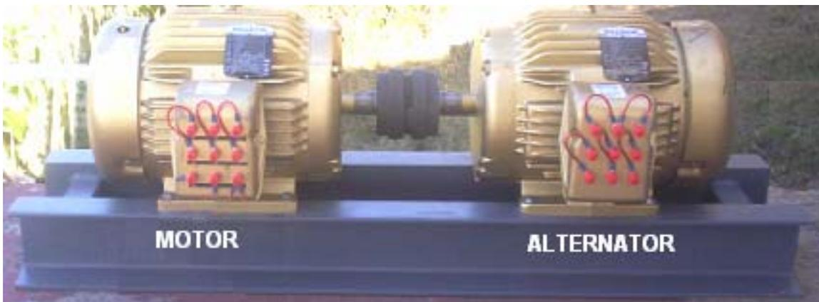
The input drive may be from an inverter driven from a battery charged via a solar panel. The system now needs to be 'tuned' and tested. This involves finding the best 'starting' capacitor which will be switched into the circuit for a few seconds at start-up, and the best 'running' capacitor. Help and advice is readily available from the EVGRAY Group as mentioned above.
