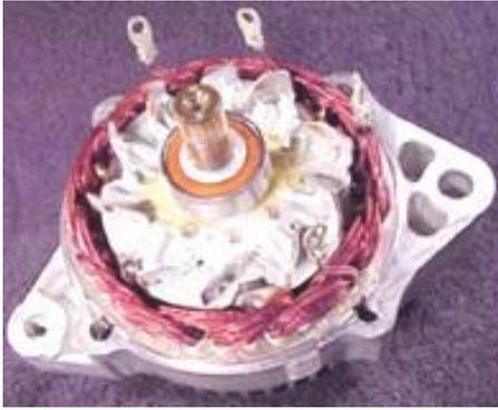
As the rotor assembly rotates within the stator winding: The alternating magnetic field from the spinning rotor induces an alternating voltage into the stator winding. The strength of the magnetic field and the speed of the rotor affect the amount of voltage induced in the stator.
