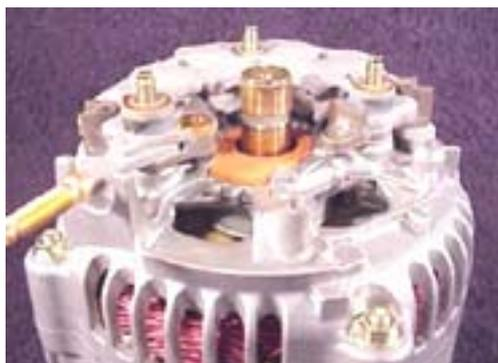
Two stationary carbon brushes ride on the two rotating slip rings. These brushes are either soldered or bolted in position.
