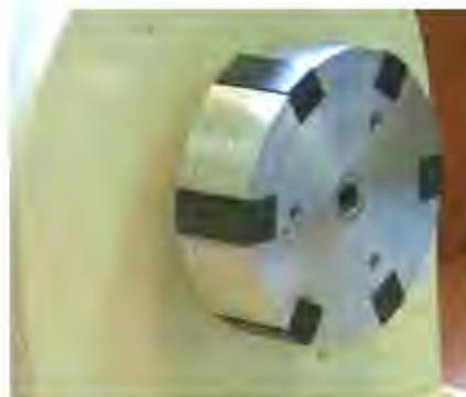
It is not desirable to recess the magnets or place a restraining layer around the circumference of the rotor as the clearance between the magnet faces and the coils needs to be as small as practical. The North poles of the magnets face outwards as shown in the diagram above. If desired, the attachment of the magnets can be strengthened by the addition of blank side plates to the rotor which allows the magnet gluing to be implemented on five of the six faces of the magnet pairs:
