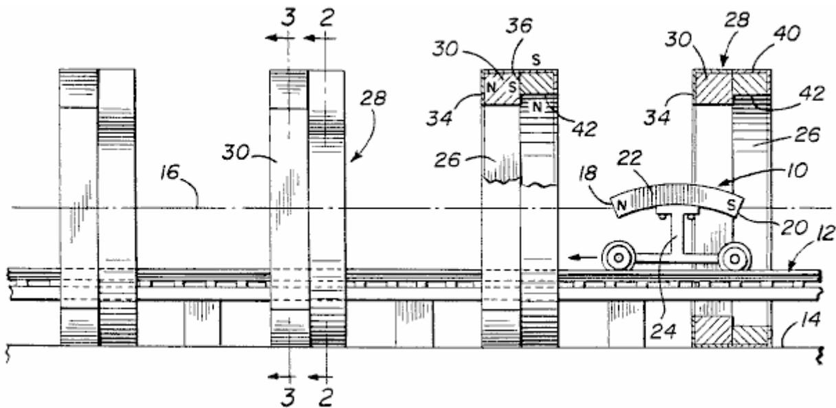
Howard demonstrates the force by placing miniature railway tracks inside the magnet rings and showing that a wheeled carriage is pushed along the tracks.
