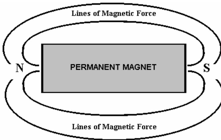
This is deduced by scattering iron filings on a sheet of paper held near the magnet. Unfortunately, that is not a correct deduction as the iron filings distort the magnetic field by their presence. More careful measurement shows that the field actually produced by a bar magnet is like this:
