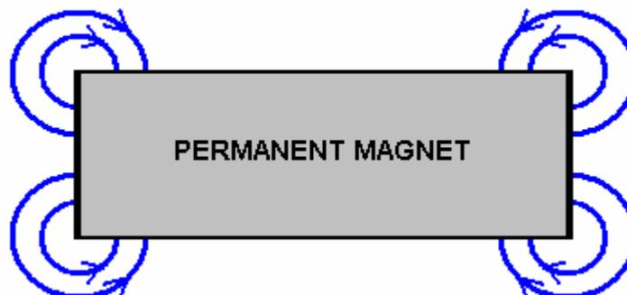
There are many lines of force, although the sketches shown above only show two. The important factor is that there is a circling field at each corner of the magnet.
