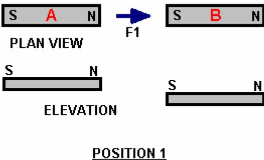
Magnet 'A' is held in a plane slightly higher than magnet 'B' so that they do not touch if they pass each other. There are four forces acting in this position:
