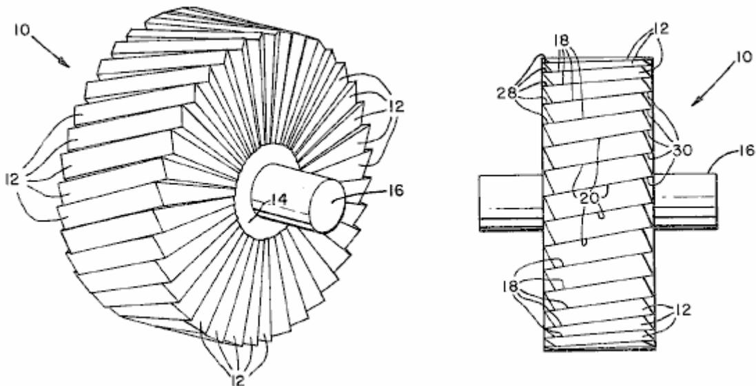
Some people have opted for permanent magnet motors where the field is shielded at the appropriate moment by a moving component of the motor. For example, Robert Tracy was awarded US Patent Number 3,703,653 on 21st November 1972 for a "Reciprocating Motor with Motion Conversion Means". His device uses magnetic shields placed between pairs of permanent magnets at the appropriate point in the rotation of the motor shaft:
