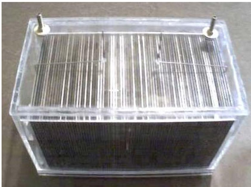
The case is constructed from perspex. The gas output is taken from either nipple with the other one capped. The electrical input is via the wires led through the middle of the top of the case. Not all electrolyzers are built this way.
