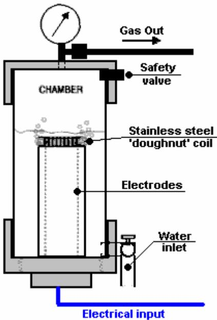
It is suggested that you use a section of 4" PVC waste pipe with a threaded screw-cap fitting on one end and a standard
