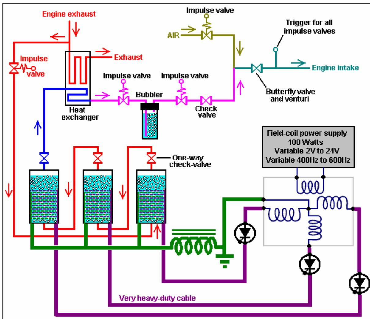
Peter uses a GEC delta-wound, marine alternator which he modifies by removing the diodes and leading each of the three phase-windings out to his electronics. He uses each of the three phase-windings to power one electrolysis cell. As he only wants about 1.5 volts across each cell, he applies about 2 volts to the DC winding of the alternator, which is about the minimum for the alternator to work.
