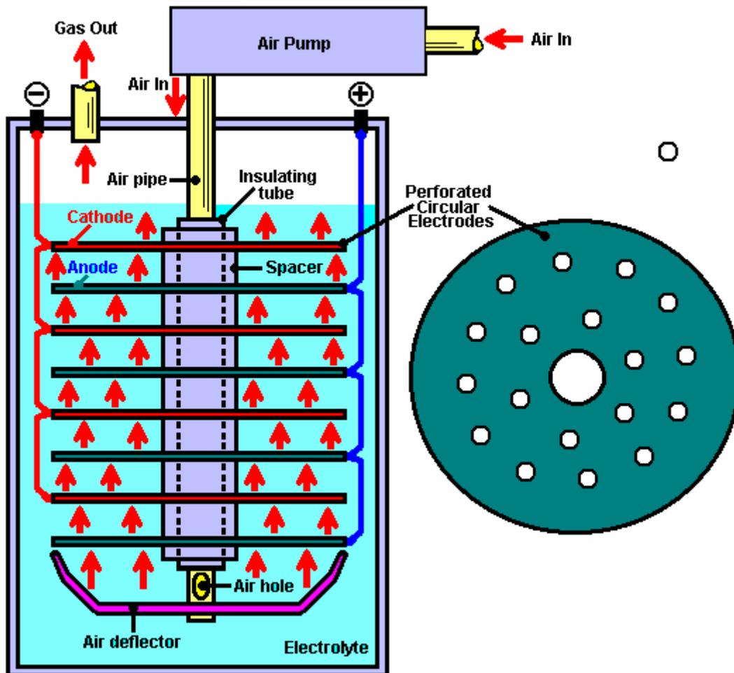
With this unit, air is sucked out of the exit pipe by the vehicle engine. This draws air down the central pipe and forces it up through the non-aligned holes in the electrode plates. The air bubbles stir the electrolyte into vigorous motion, dislodging the hydrogen and oxygen bubbles which form on the plates through electrolysis.
