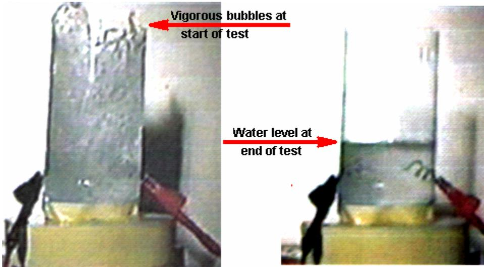
This is said to split one litre of water per minute in a single cell with just bare wires for the electrodes and a straight square wave between the electrodes. He used 10% sulphuric acid solution (probably unnecessary). Anode and cathode were 35 mm (1.4 inch) long, silver-coated copper wire. Paulo ran his internal combustion lawnmower directly from water using this method:
