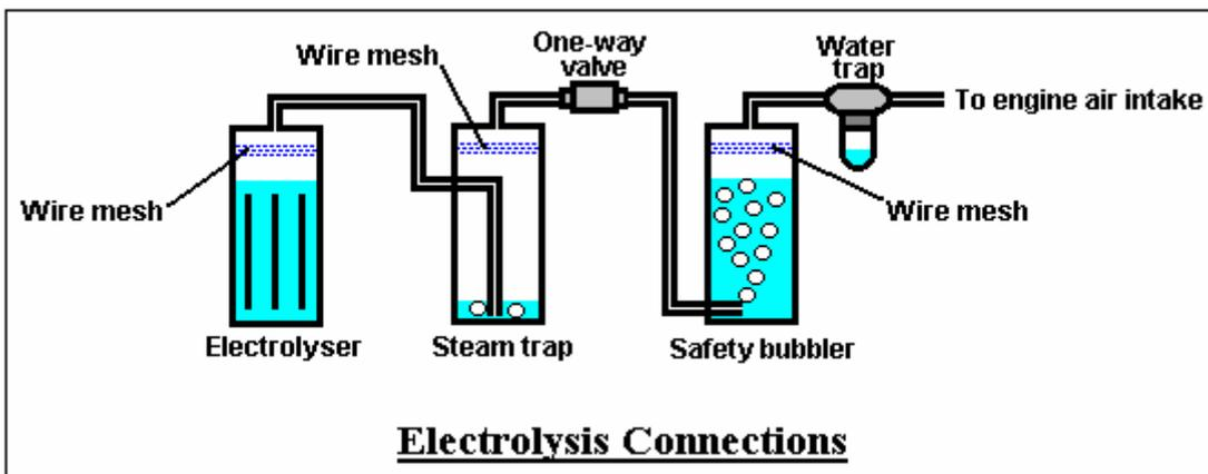
The bubbler also has stainless steel wire mesh screens which the gas has to pass through before it exits the bubbler. The gas is then passed through a compressor-style water trap to remove any remaining moisture, and is injected into the air intake of the vehicle. Although not shown in the diagram, the containers are protected by pop-out fittings which provide extra protection in the extremely unlikely event of any of the small volumes of gas being ignited by any means whatsoever.
