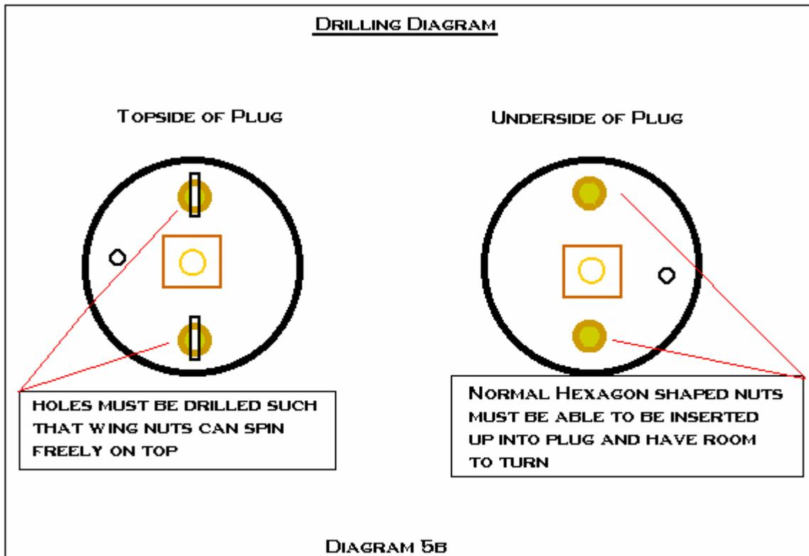
Use a red indelible marker to designate one of these holes as the positive terminal. Drill a hole in the top of the raised square on the plug such that the threaded hollow rod can be threaded into it. Drill a 1/8 inch 'bleeder hole' (as in diagram 5a) in the top of the cap on the side of the square that has not already been drilled through. This bleeder hole acts as an air intake for the pump to operate with.
