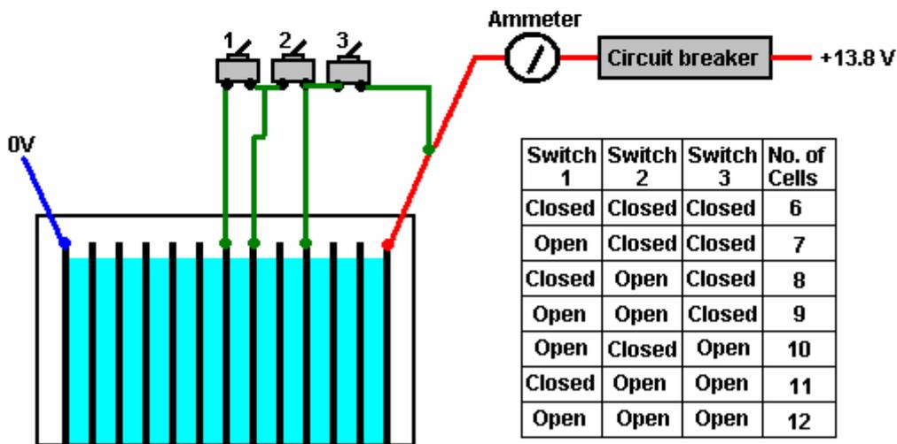
In the first option, the arrangement is very simple with three switches adding in three additional cells - one switch per cell, very easy to understand and operate. The second arrangement uses the same three switches but it allows twice as many extra cells to be switched in. However, the switching arrangement is more complicated when driving along with one switch having to be opened and another having to be closed.
