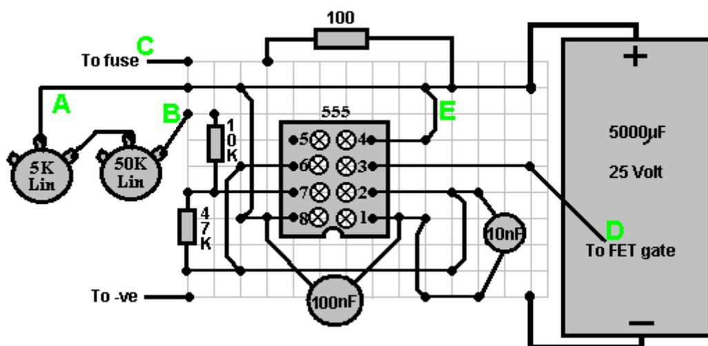
The jumper from pin 4 of the 555 chip (point 'E') which is shown going to the positive line, would instead be taken to the on/off switch of the gating 555 if gating is used.
