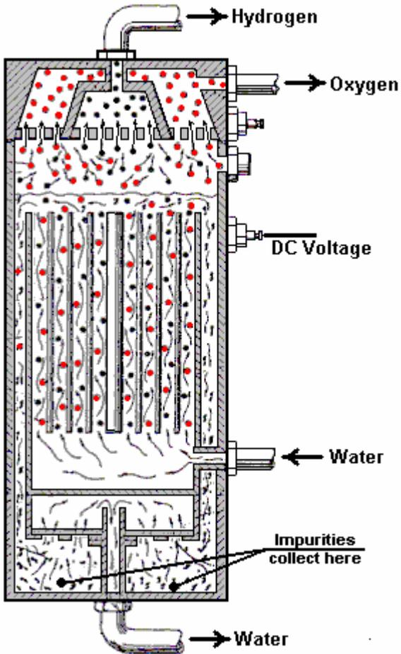
You will note that he uses a DC voltage on the wall of the cell to move the dissociated hydrogen atoms outwards and the oxygen atoms inwards, to produce separate gas exits from the cell.
