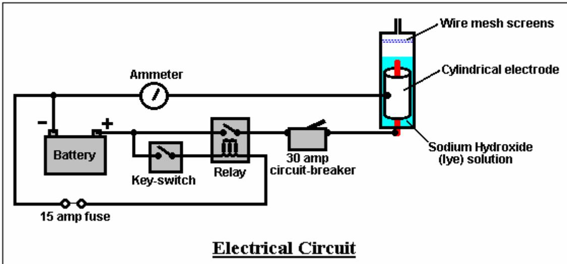
The circuit is wired so that it is only powered up when the car ignition switch is closed. A relay feeds power to the electrolyser which is three inches (75 mm) in diameter and about 10 inches (250 mm) tall. The electrolyser circuit is protected by a 30-amp circuit breaker. The electrolyser has several stainless steel wire mesh screens above the water surface.
