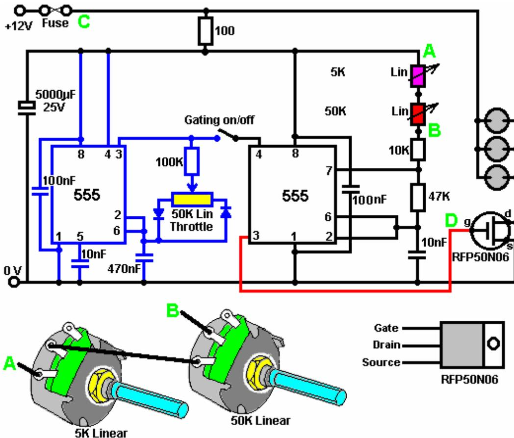
This is just a crude circuit which could easily be improved by giving the 555 chips a stabilised and/or smoothed power supply of say, 9 Volts or so. The gating part of the circuit is marked in blue and is optional - Paulo Mateiro did not use one and claimed spectacular gas production.
