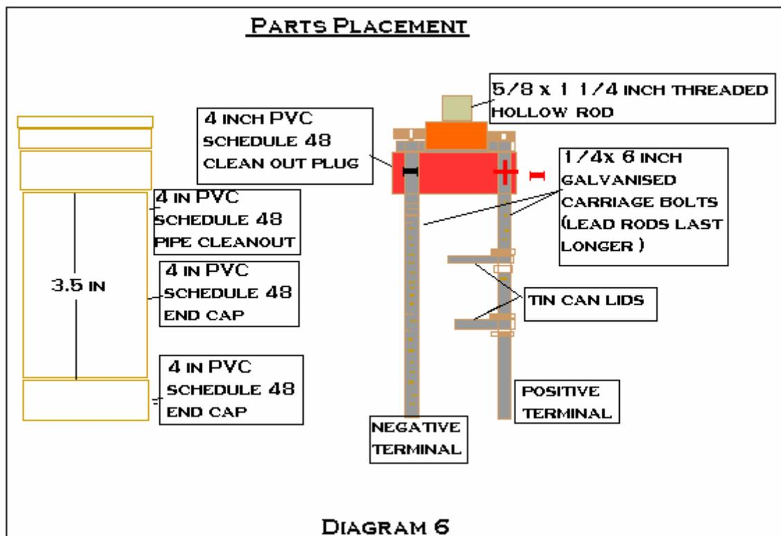
Also drill many holes in these lids such that a grid pattern is produced (these holes may also be made by using a nail to punch through the lids), hydrogen bubbles will form around the perimeters of all of these holes. Since these lids give the hydrogen more edges to collect on, a greater volume of hydrogen seems to be produced. I tried using more than two plates and found the amount of hydrogen did not seem to increase further.
