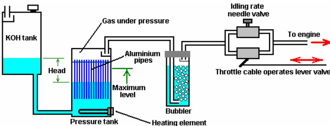
Here, there is a header tank containing a 25% mixture of Potassium Hydroxide (KOH) in water. This tank is positioned higher than the pressure tank where the hydrogen gas is generated and the venting pipe is protected by a baffle. The
