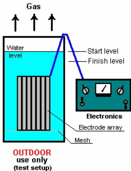
Fill the container to the upper mark, start the experiment and measure the length of time it takes for the water level to fall to the lower mark. It is much easier to measure the loss of water than to capture the gas and measure its volume and pressure.
