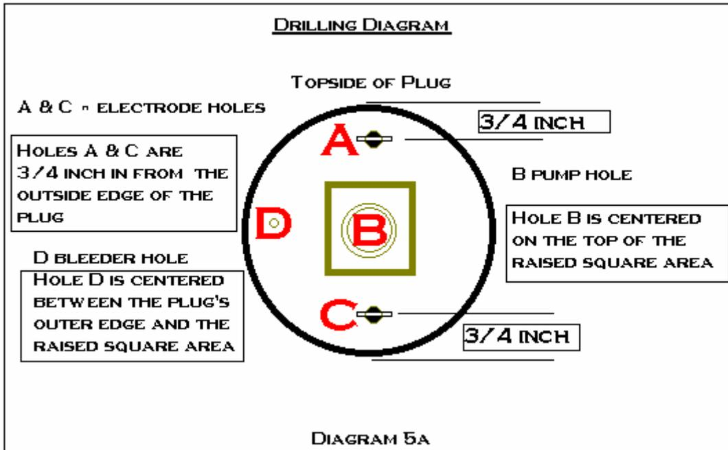
Refer to Diagram 5a and drill holes on either side of the square raised area on the PVC plug that will allow the carriage bolts to be threaded into the holes. But take care that the hole is far enough in so that a nut affixed to the bolt will be able to fit into the underside of the plug without getting caught on its rim. (see Diagram 5b).
