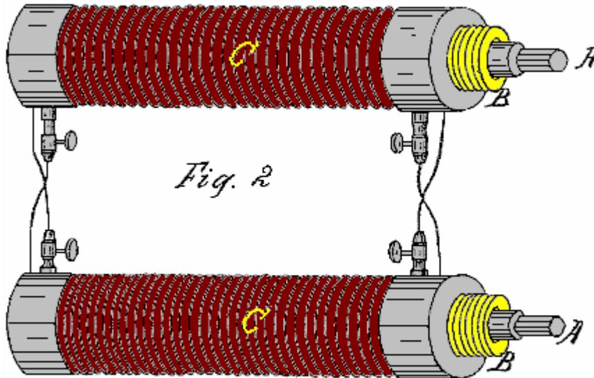
In carrying out my invention, I do not confine myself to any particular mode of coil construction or to any particular size of wire, observing only that the quantity of wire in the various coils must be sufficient to produce the required result; also, the material used to insulate the wires must be suitable for producing the required result. However, I generally prefer to use the same size of wire in the construction of both simple and compound coils.
