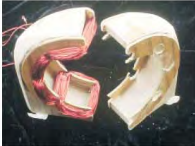
The two stator halves—one wound with 100 turns per coil, and one ready to be wound.
