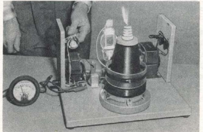
After you finish the assembly, read the plate current by connecting a D.C. milliammeter between the center tap of the filament transformer and ground. Adjust the rheostat to 150 ma. maximum for any combination of capacitors and taps
